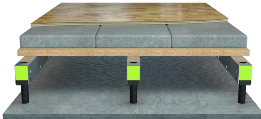
Figure 3: Picture of the floating slab. In cinemas the upper board was chipboard and a layer of glass wool was placed in the cavity below the floor.
